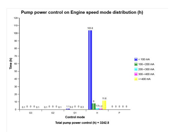
The diagram describes the distribution of pump power control current operation on each engine mode
