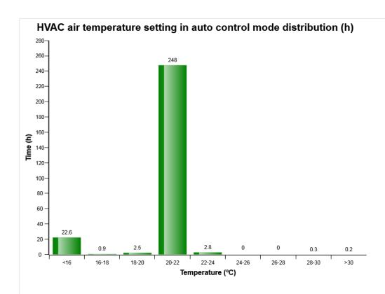
The diagram describes air temperature setting distribution for HVAC auto control mode established by operator in Cabin
