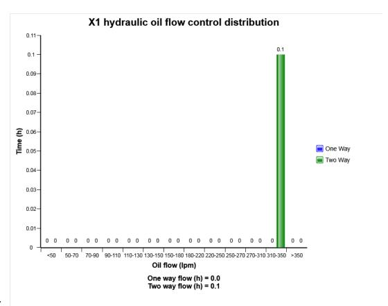
The diagram describes X1 hydraulic oil flow control distribution of the machine while machine operates.
