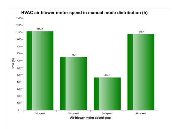
The diagram describes air blower motor speed distribution for HVAC manual control mode established by operator in Cabin.
