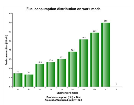
This diagram shows the fuel consumption distribution rate on each work mode.
