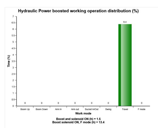
The diagram describes Power boosted operating time distribution, when main relief pressure increases on working operation modes. In this diagram, the sum of time (%) of each working operation mode can exceed 100%. It means that customer has been operated several working operations at the same time.
