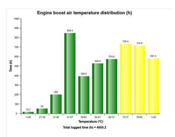
The diagram describes Engine boost air temperature distribution of the machine when the engine is on.
