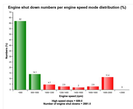
The diagram shows the number of stops at high idle (I1 ~ P mode).
