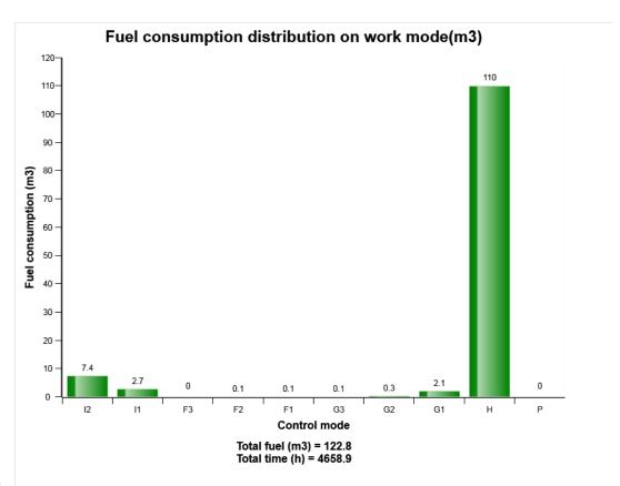
The diagram describes the amount of fuel consumed per engine speed mode distribution.
